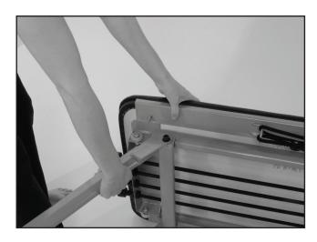
Turn the platform upside down so it is cord side up. Using a crescent wrench and flat head screwdriver, remove the screw that is holding the roller in place. Replace the old roller with the new one, add the washer, push the screw through the roller and tighten with the nut. Do not overtighten the nut and make sure the roller turns easily.
