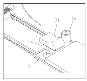
Make sure that both FOAM PADS(16) are in the PLATFORM(7) when using the HEAD & NECK SUPPORT PILLOW(71) attached to the HEADREST(14).
