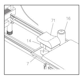
Make sure that both FOAM PADS(16) are in the PLATFORM(7) when using the HEAD & NECK SUPPORT PILLOW(71) attached to the HEADREST(14).
