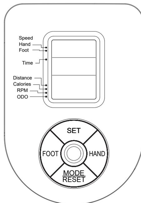
**NOTE:** The meter is designed to show the function values of HAND and FOOT separate, except the TIME. The Time function will show when both the handlebar and pedaling are moving together.
