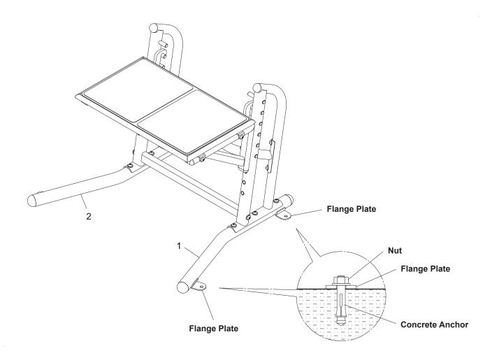
**NOTE:** Four concrete anchors (mounting hardware not included) are needed to secure the **RIGHT** and **LEFT BASES(1, 2)** of the **Stamina® Outdoor Fitness Adjustable Plyo Box**, two on each side.
