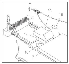
Make sure that both FOAM PADS(16) are in the PLATFORM(7) when using the HEAD & NECK SUPPORT PILLOW(59) attached to the HEADREST(14).
