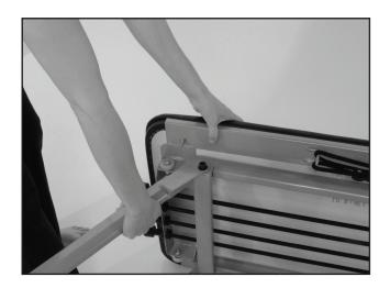
Turn the platform upside down so it is cord side up. Using a crescent wrench and flat head screwdriver, remove the screw that is holding the roller in place. Replace the old roller with the new one, add the washer, push the screw through the roller and tighten with the nut. Do not overtighten the nut and make sure the roller turns easily.
