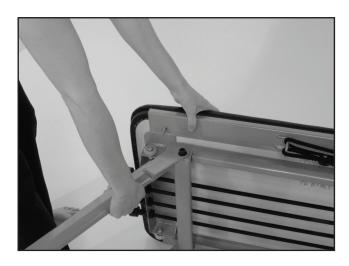
Turn the platform upside down so it is cord side up. Using a crescent wrench and flat head screwdriver, remove the screw that is holding the wheel in place. Replace the old wheel with the new one, add the washer, push the screw through the wheel and tighten with the nut. Do not overtighten the nut and make sure the wheel turns easily.
