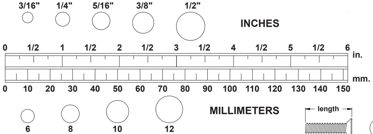
**NOTICE:** The length of all bolts and screws, except those with flat heads, is measured from below the head to the end of the bolt or screw. Flat head bolts and screws are measured from the top of the head to the end of the bolt or screw.
