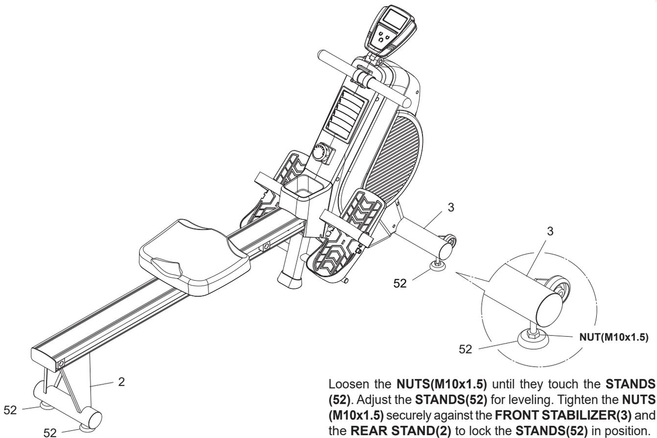
Loosen the **NUTS(M10x1.5)** until they touch the **STANDS (52)**. Adjust the **STANDS(52)** for leveling. Tighten the **NUTS (M10x1.5)** securely against the **FRONT STABILIZER(3)** and the **REAR STAND(2)** to lock the **STANDS(52)** in position.
