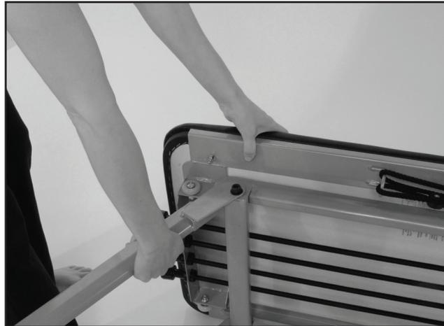
Turn the carriage upside down so it is cord side up. Using a crescent wrench and flat head screwdriver, remove the screw that is holding the wheel in place. Replace the old wheel with the new one, add the washer, push the screw through the wheel and tighten with the nut.
