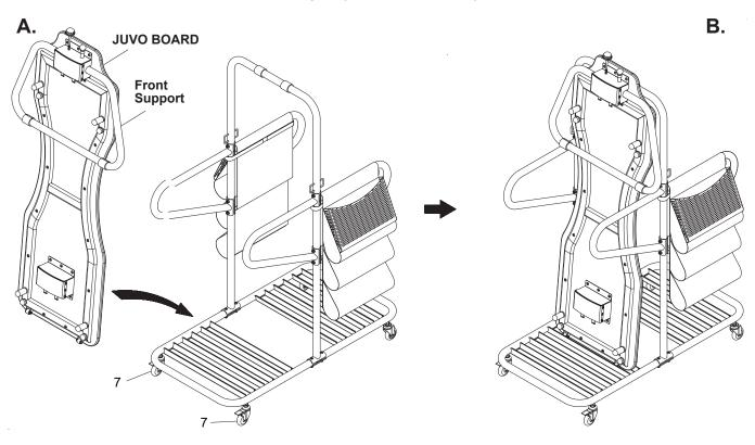
The JUVO BOARD CART stores a maximum of six JUVO BOARDs as shown in the illustration. Secure the JUVO BOARDs to the JUVO BOARD CART with the STRAPS(8). Pull the STRAP(8) through the Front Support to ensure a snug and safe fit. The STRAP(8) can be clipped to far side hook for a tighter fit.
