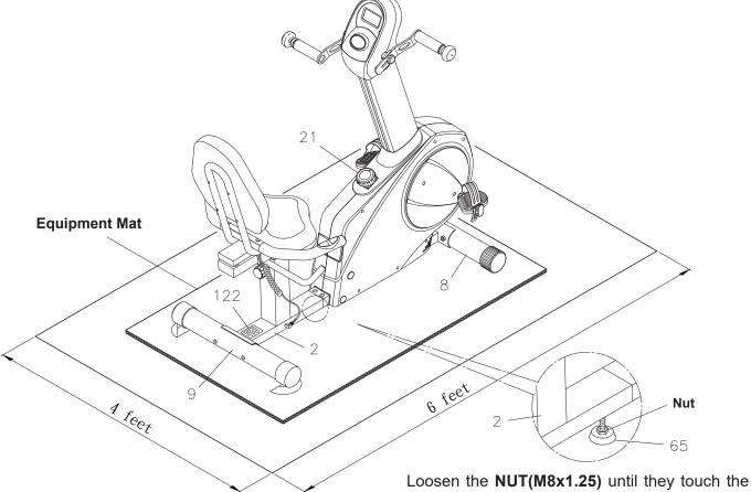
Loosen the **NUT(M8x1.25)** until they touch the **LEVELING STAND(65)**. Adjust the **LEVELING STAND(65)** for leveling. Tighten the **NUT (M8x1.25)** securely against the **REAR FRAME(2)** to lock the stand in position.
