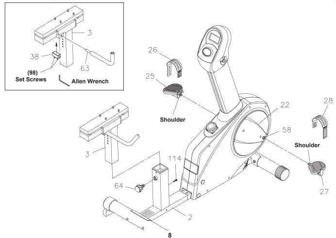
**NOTE:** Be careful not to damage the **PULSE SENSOR WIRES(104)** while doing assembly Step 8 and Step 9.
