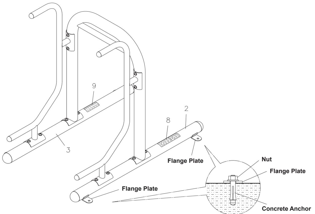
**NOTE:** Four concrete anchors (mounting hardware not included) are needed to secure the **LEFT** and **RIGHT BASES(2, 3)** of the **STAMINA® Outdoor Multi-Station**, two on each side.
