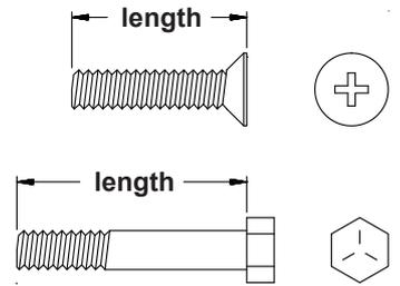
**NOTICE:** The length of all bolts and screws, except those with flat heads, is measured from below the head to the end of the bolt or screw. Flat head bolts and screws are measured from the top of the head to the end of the bolt or screw.
